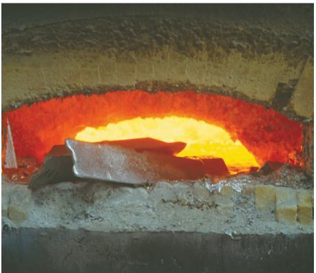
Continuous and dedicated design is needed to obtain strong, light and elegant products. The production of aluminium radiators begins with the smelting in automated ovens of ingots of aluminium alloy EN AB 46100.
