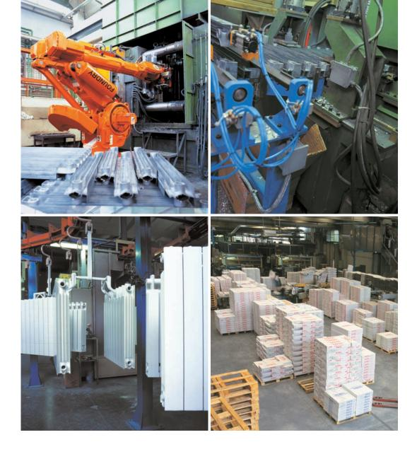
The liquid aluminium is passed to waiting furnaces from which the injection moulding machines are fed automatically.
