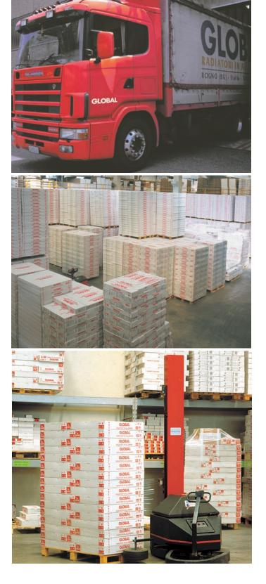
Finally, all radiators are enclosed in a polythene film and packed in a strong export carton to protect them up to the moment of installation.
